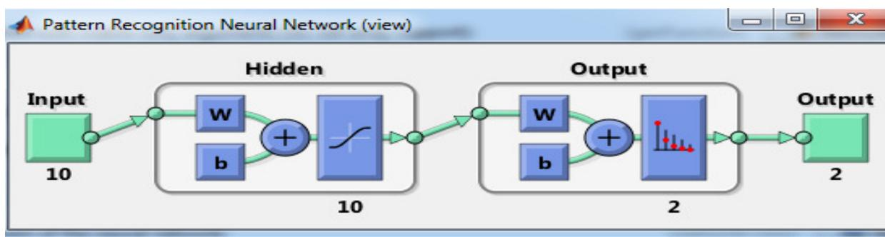
**Fig. 16. Two-Layer Feed Forward Neural Network.**
